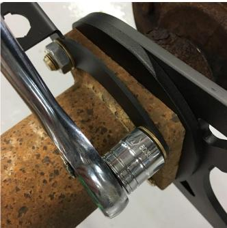
**For standard, low-offset kits:** The bracket and hardware will sandwich the .25" spacer as shown. **For high-offset kits:** use the machined aluminum spacers in place of the .25" spacer. It will need to be installed with the counterbore facing the flange. In order to do this the axle will need to be removed from the housing.
