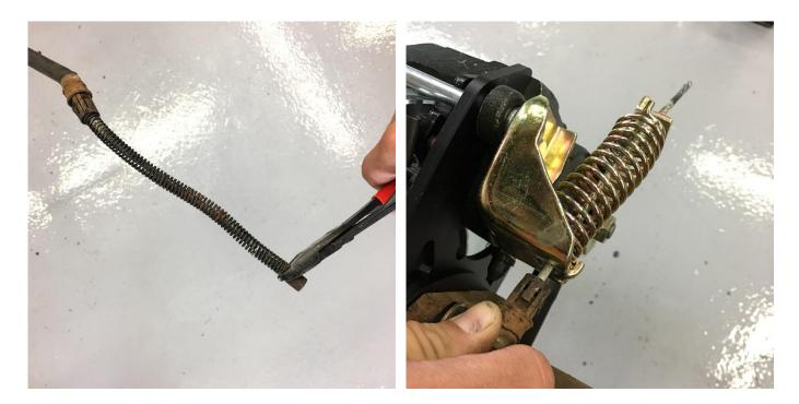
Depending on factory cable lengths, the existing cables can sometimes be used without any modification. If they are too long, then cut off the cable stop as shown using cable cutters or a cut-off wheel. The spring can be removed with the cable installed into the parking brake caliper as shown.
