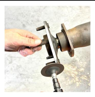
**Normally not required**, **but for some 5-lug kits and 5.1" offset 6-lug kits**, the OD of the axle shaft flange may be too large to fit inside of the supplied rotor. If this happens, the solution is to simply remove material from the outside of the axle flange with a sander while rotating the shaft as shown.
