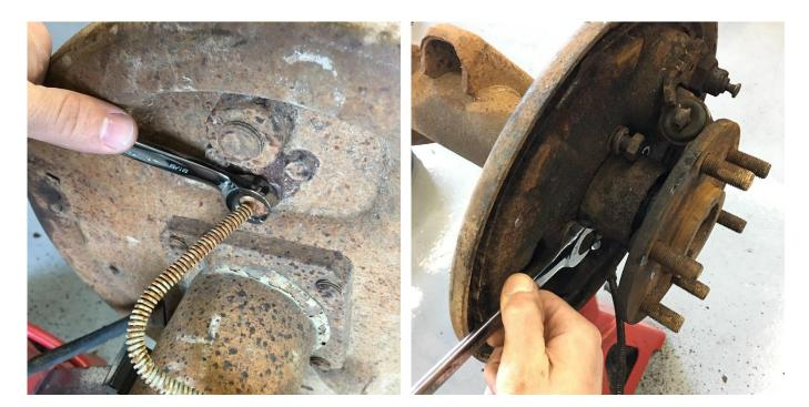
Remove the brake line from the wheel cylinder using a line wrench if possible. The 4 bolts retaining the drum backing plate to the axle can now be removed and discarded.
